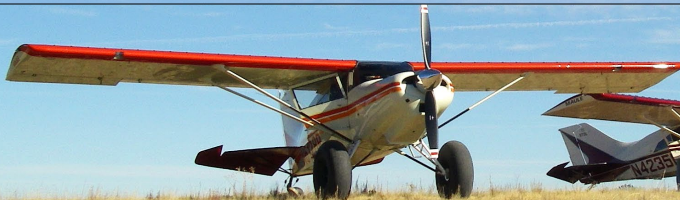
M-7-235A with Oleo Strut Main Gear
