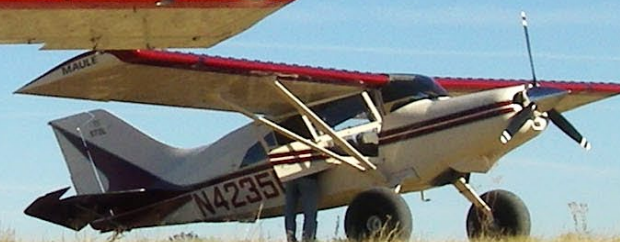
M-7-235C with Aluminum Spring Main Gear
