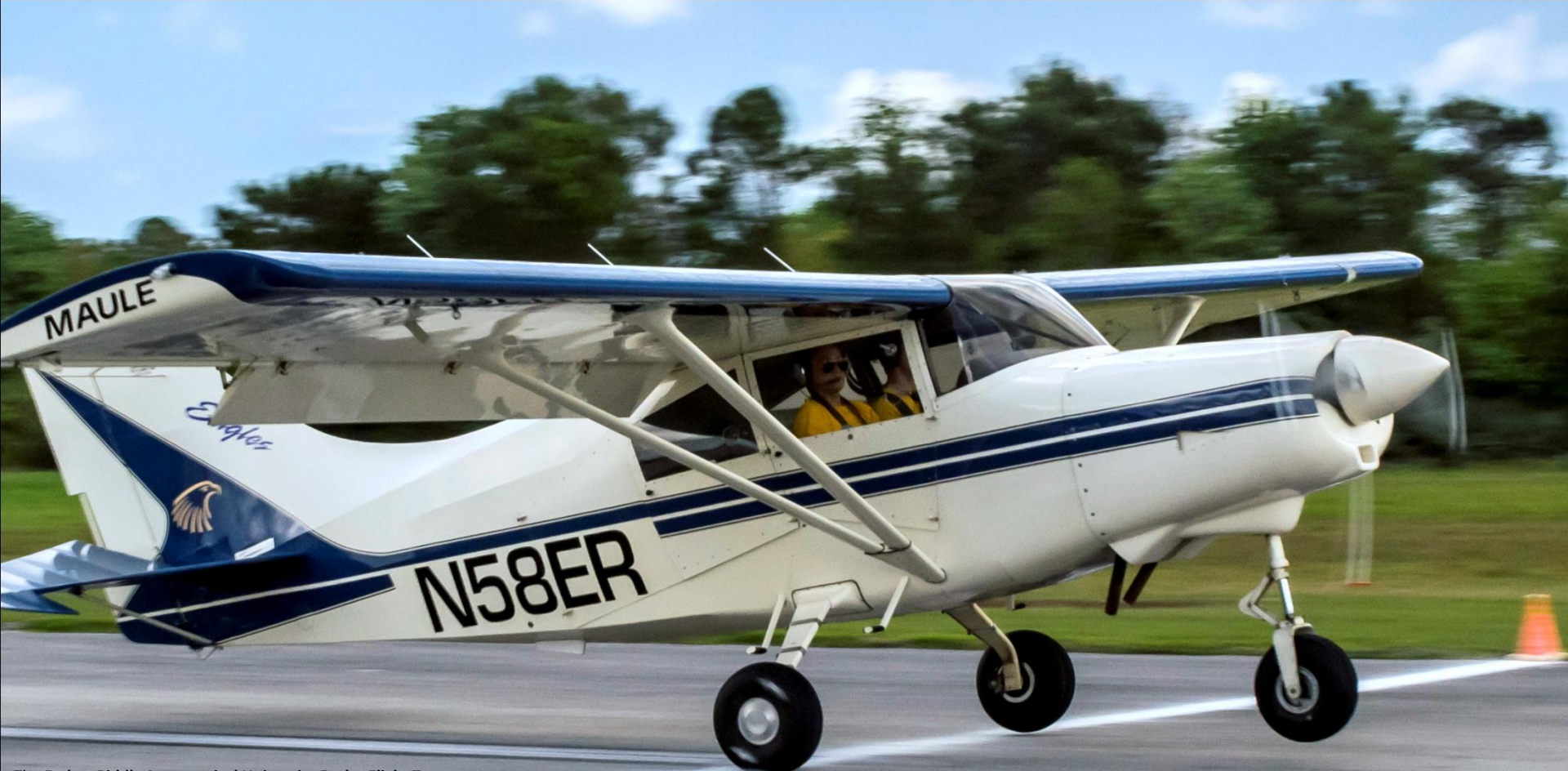
The Embry-Riddle Aeronautical University Eagles Flight Team Spot Landing in a MAULE MXT-7 with a 180 hp O-360 Lycoming Photos courtesy of J. C. Swain
