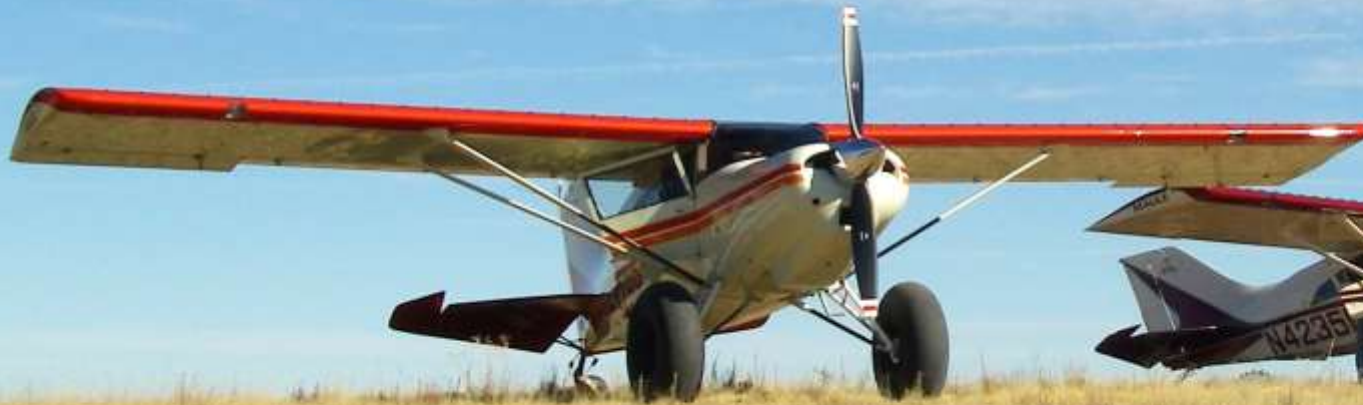
MAULE M-7-235A with Oleo Strut Main Gear
