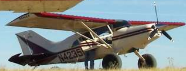
MAULE M-9-235 with Aluminum Spring Main Gear
