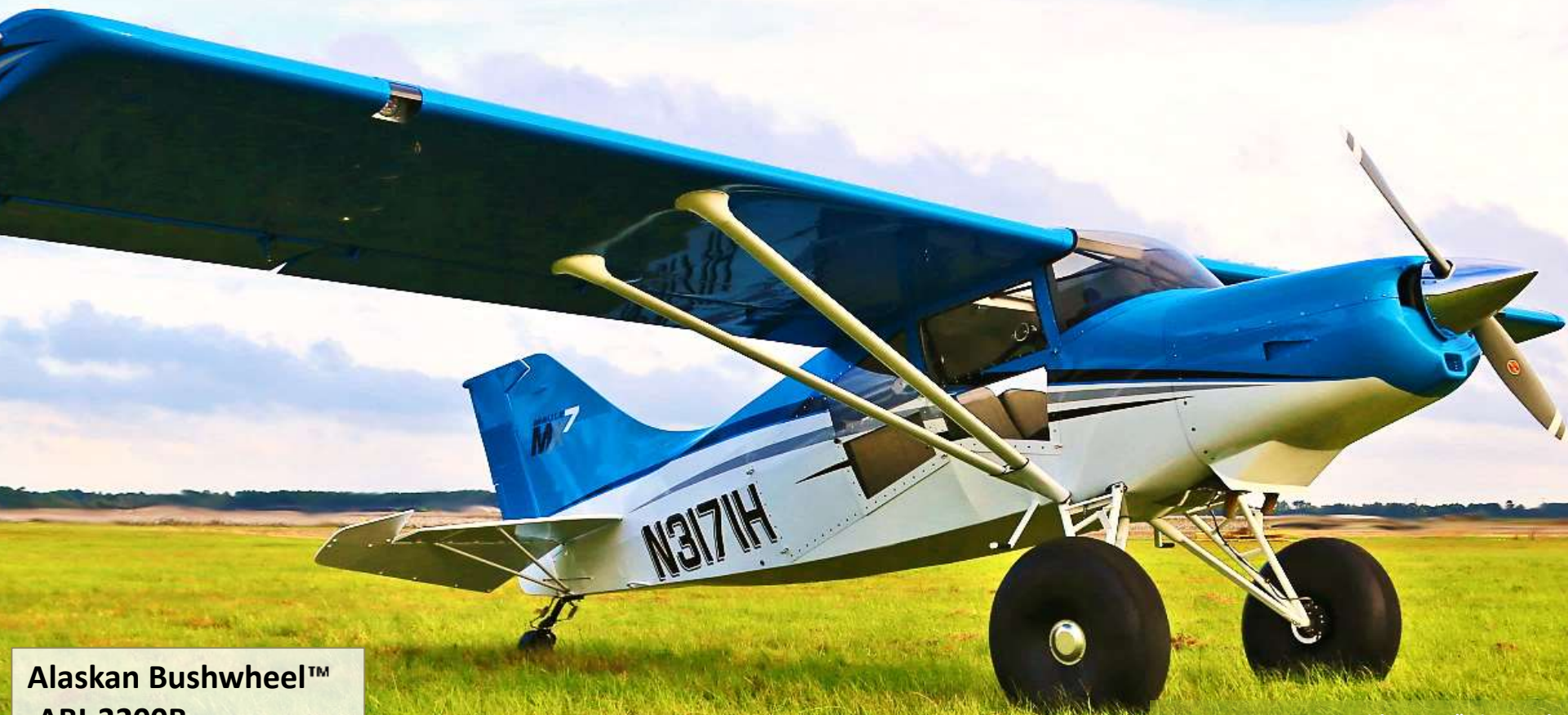
MAULE MX-7-180B with ABI 31" Tires and 4" Extended Landing Gear
